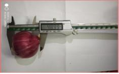
**Fig. 1.** Polar diameter  $(D_p)$ .
